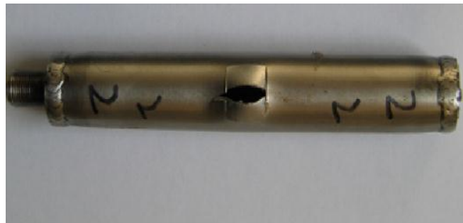
Figure 10: Maximum strain at the middle of local wall thinning area, Hui and Li SG 690 tube experiment [3]
